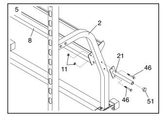
6. Press a 25mm Round Inner Cap (51) into the end of the other Weight Storage Tube (21).
